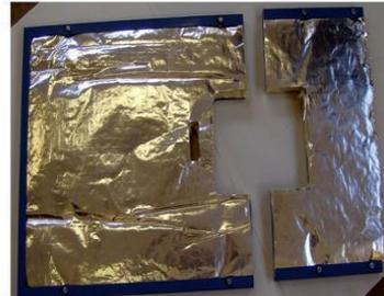
Drape the large piece of block insulation directly over the block taking care to provide adequate clearance from frame rails. Using the aluminum faced tape attach the pre-shaped rear insulation to the block insulation. The process is simply taping the two pieces together. The front panels come pre-insulated.
