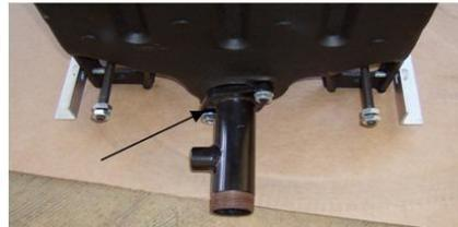
Using the gaskets and bolts supplied connect the manifolds directly to the boiler block. The top supply manifold will have a 3/4 in. npt tapping for a relief valve and a 1/4 in. npt tapping for a gauge. The bottom return manifold has a 3/4 in. npt tapping for a drain valve. Both manifolds have 1 1/4 in. male npt threads for system connection.
